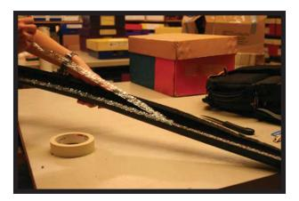
3) Place masking tape all along the edge with the sticky stuff—press the tape down firmly so you know it's stuck. Then pull the tape off to remove the sticky stuff. Now your pipe insulation is ready!
